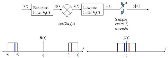
(b) The first **discrete-time signal processing block** is filtering. Design a **second-order** linear time-invariant (LTI) infinite impulse response (IIR) filter to extract channel k from y[n]. Assume the sampling rate in part (a) is  $f_s = 200$  MHz. Give formulas for, and plot, the two poles and two zeros. *9 points*.
