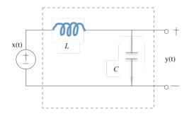
The initial voltage across the capacitor is 0 V and the initial current in the inductor is 0 A; hence, the circuit is a linear time-invariant system.
